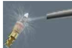
Sandblast the bonding surface
