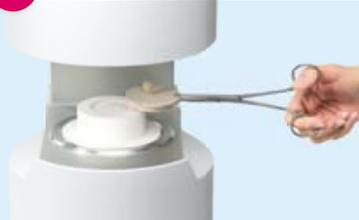
Remove the firing tray and restoration
