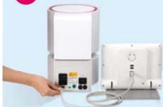
Connect the firing unit and control unit with the connection cable.
